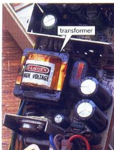
A small transformer with other components from inside a TV
